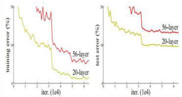
Fig 6: Training error (left) and test error (right) on with 20-layer and 56-layer “plain” networks. The deeper network has higher training error,
